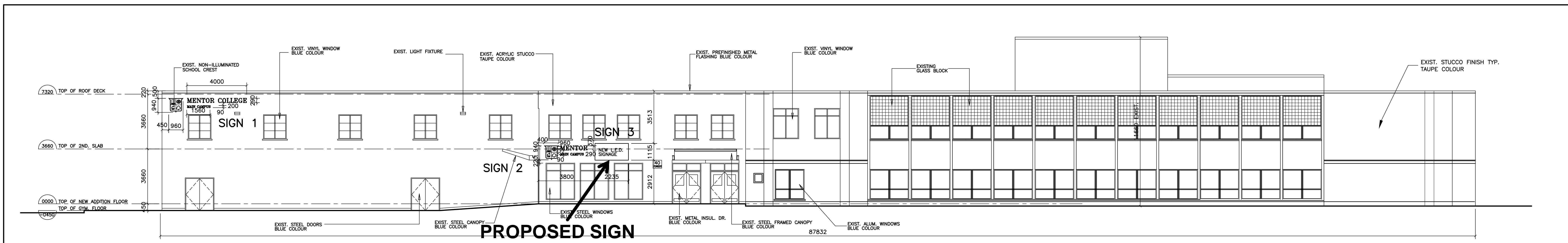
4 EXISTING SOUTH ELEVATION UNCHANGED WALL AREA: 687.72 S.M. TOTAL SIGN AREA: 5.78 S.M. = 0.84 % OF WALL AREA A4 SCALE: 1:100
